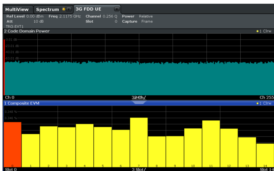
Figure 10-7: Measurement Example 5: Measuring the Composite EVM
